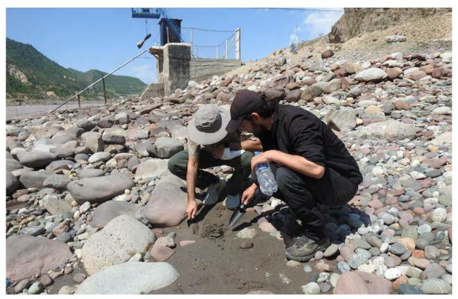
MSRI Scientists collecting sediment samples from the Vakhsh River as part of the World Bank funded project to study sediment loads to Nurek Dam, the largest hydropower station in Tajikistan.
